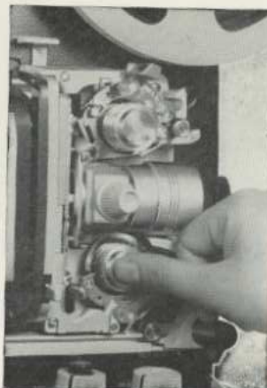
Push the lower sprocket shaft for using Regular 8mm film.
