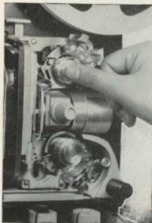
Push the upper sprocket shaft for using Super-8 size film.
